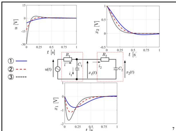
(2)  $A = \begin{bmatrix} -2 & 0 \\ 0 & -2 \end{bmatrix}, B = \begin{bmatrix} 2 \\ 0 \end{bmatrix} \quad u(t) = kx(t) = \begin{bmatrix} k_1 & k_2 \end{bmatrix}$
