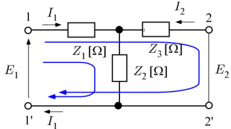
$$Y_{11} = \left[ \frac{I_1}{E_1} \right]_{E_2=0} = \frac{1}{Z_1 + \frac{Z_2 Z_3}{Z_2 + Z_3}} = \frac{Z_2 + Z_3}{Z_1 Z_2 + Z_2 Z_3 + Z_3 Z_1}$$
