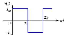
$$b_n = \frac{1}{\pi} \int_0^{2\pi} f(t) \sin n\omega t dt \\ = \frac{1}{\pi} \left( \int_0^{\pi} I_m \sin n\omega t dt + \int_{\pi}^{2\pi} (-I_m) \sin n\omega t dt \right) \\ = \frac{I_m}{\pi} \left( \left[ -\frac{1}{n\omega} \cos n\omega t \right]_0^{\pi} - \left[ -\frac{1}{n\omega} \cos n\omega t \right]_{\pi}^{2\pi} \right) \\ = -\frac{I_m}{n\omega\pi} (\cos n\omega\pi - 1 - (\cos 2n\omega\pi - \cos n\omega\pi))$$
